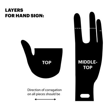
Cut these pieces out of board. It is helpful to cut the fingers all at the same time (in a stack), so they line up perfectly.
