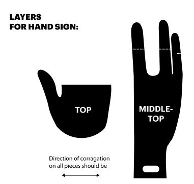
Cut these pieces out of board. It is helpful to cut the fingers all at the same time (in a stack), so they line up perfectly.
